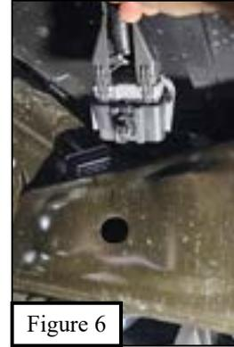
7. Detach the end of the wiring harness that is located in the inside of the bumper, see **Figures 7 & 8**.
